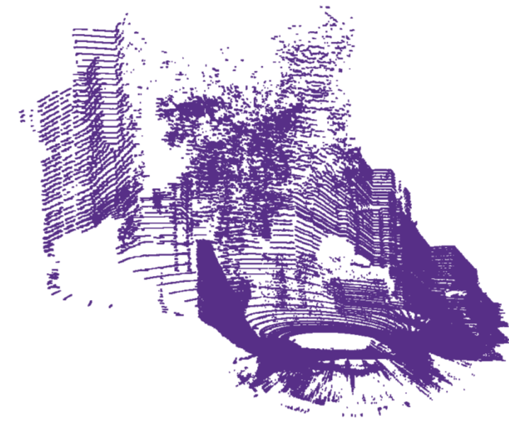
Step 1: merging the (static) background points over several frames
