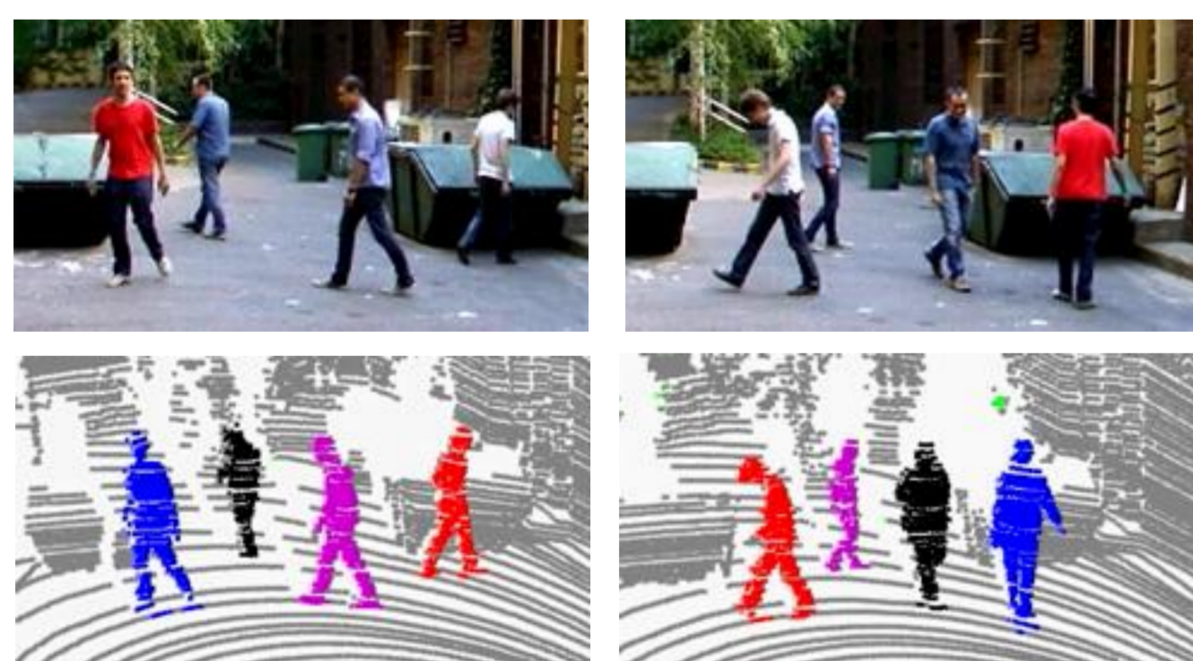
Step 3: pedestrian tracking by a Kalman filtering technique
