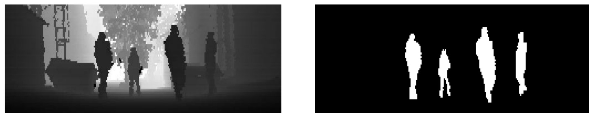
Step 1: range image formation and foreground-background segmentation by a dynamic MRF model
