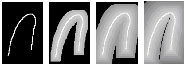
Figure 3: A simple object; and waves of dilatation after 10, 20, and 25 iterations, showing the derived symmetry axis
