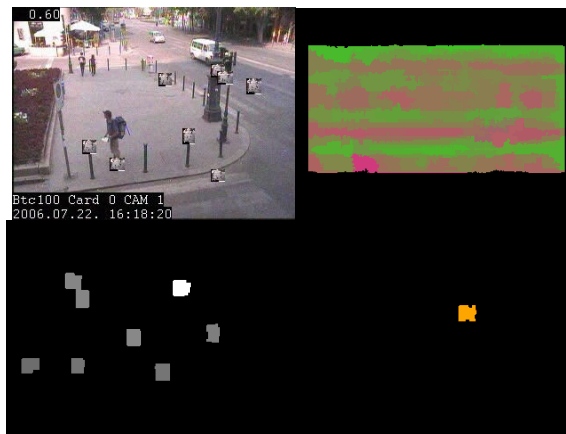
Fig. 8. A synthetic example: top-left: input frame, top-right: typical motion patterns, color coded (horizontal two-directional motions, thus the two colors), bottom-left: a screen from the learning phase where masks show the moving objects, intensity corresponds to motion speed, bottom-right: a screen from the alarm phase where a diagonally moving object is marked as unusual and an alarm is raised.
