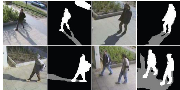
Fig.3 Examples of shadow and motion detection in real outdoor videos.
