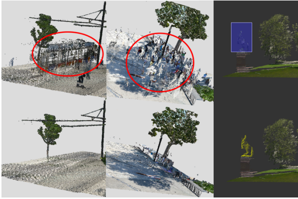
Figure 12 TLS point clouds before and after noise filtering and the annotation process on the right side
